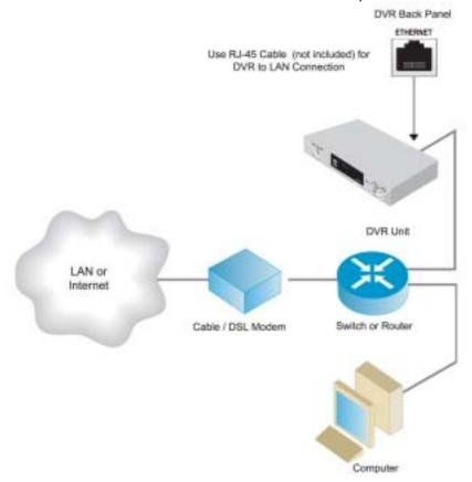
**Note:** Suitable network routers and switches are available from Net gear, D Link, or Linksys. Your internet connection requires a dedicated static IP address from your DSL provider and port forwarding capability on your router.
